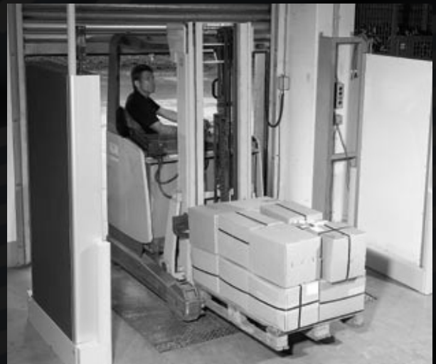
RFID enabled product being moved through demonstration gantry scanner in Europe
